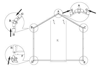
7. Secure the Rafter Poles together at the peak of the roof using Connector A. Make sure the unconnected point on the Connector faces towards you.
